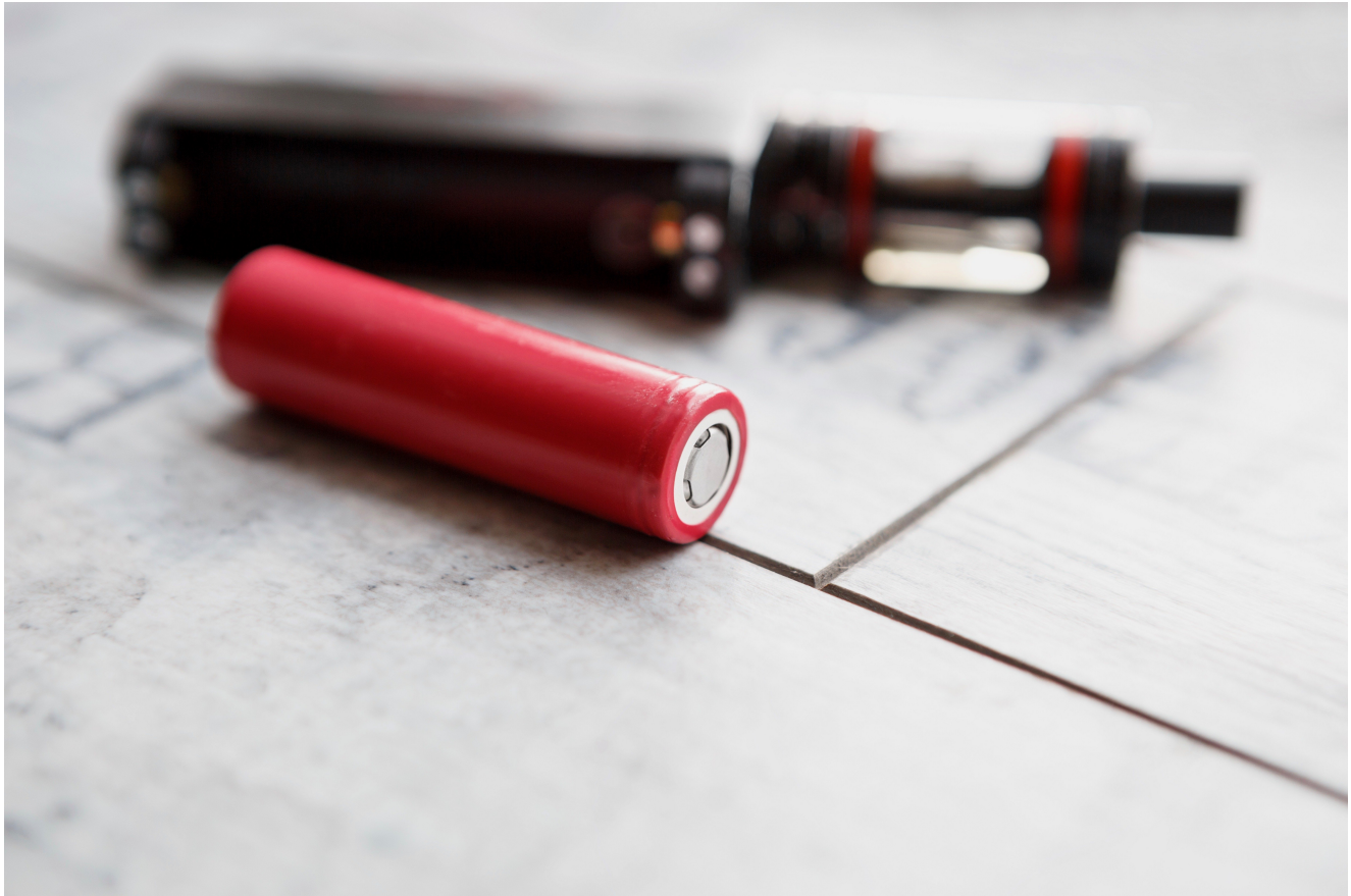
The 18650 battery is a lithium-ion variety commonly used in vape devices. Permission granted by Call2Recycle
